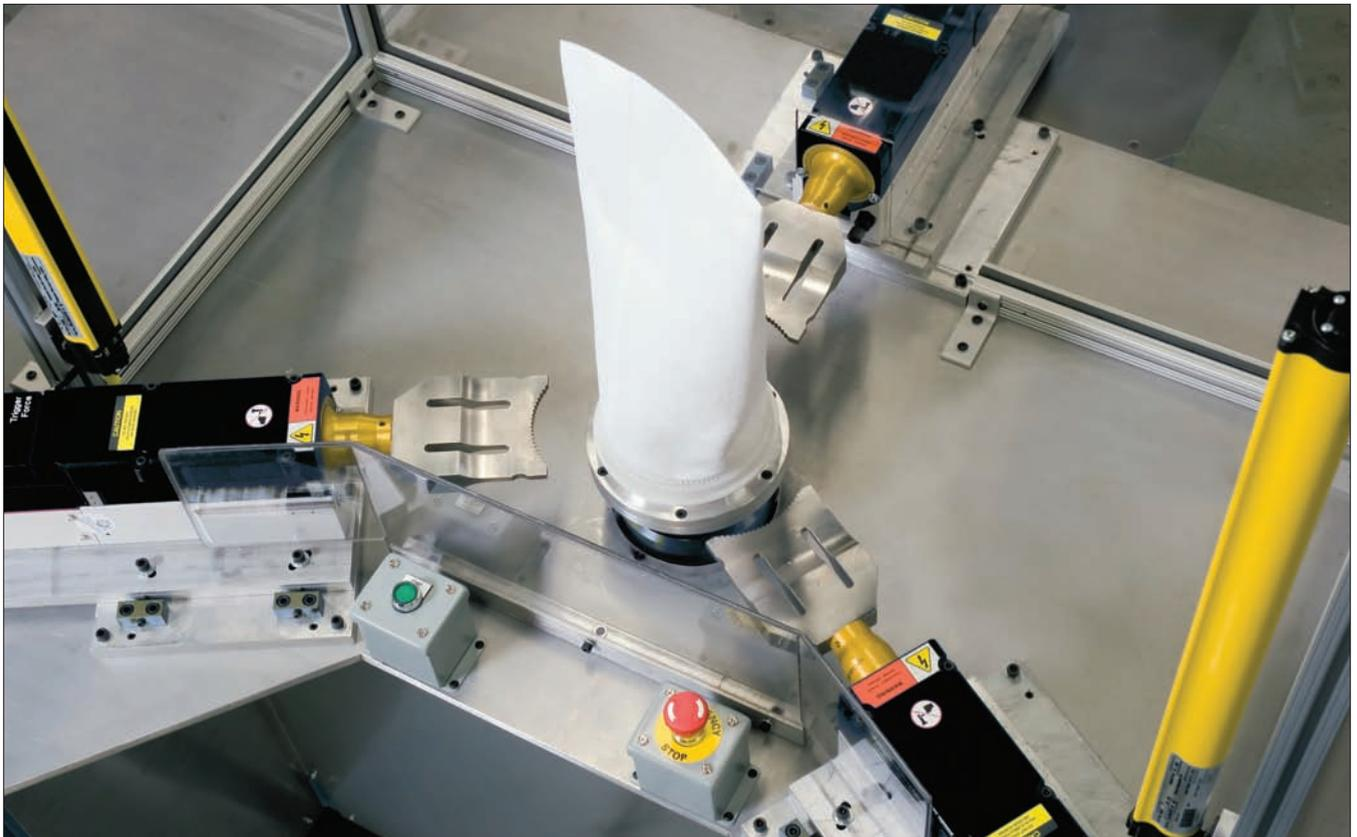
*Chase Machine and Engineering's 3-head ultrasonic ring welder provides customers the ability to attach filter bags to plastic rings without the use of needle and thread.*
